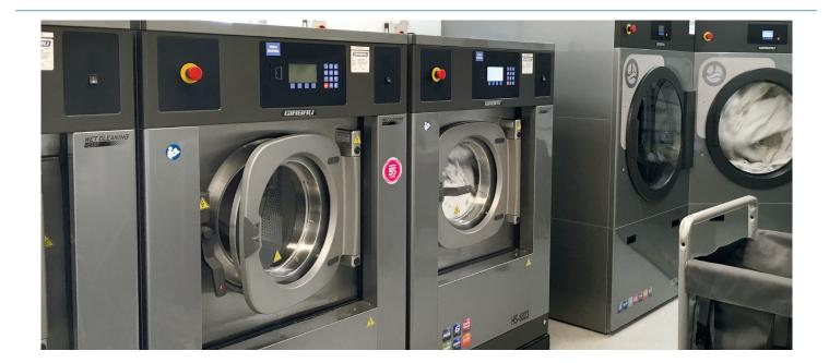
The ED660 gas dryers feature a 37 kg capacity drum, cabinet insulation, and a double-glazed door, preventing heat loss and ensuring maximum energy efficiency. Their advanced Humidity Control system detects when textiles are dry and automatically triggers the cool-down phase, reducing energy consumption and preserving fabric quality. With this system, a full 75 lb (34 kg) load dries in just 25 minutes, enhancing operational efficiency.
